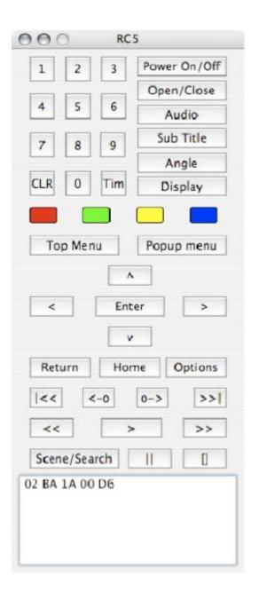
In the example to the left the key command data is 1A, the last byte is the check sum D6, these are the only two values that change when different keys are depressed.
